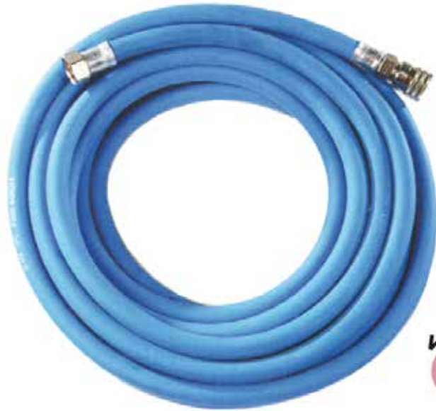
Cleaning hose, food quality, FDA approved, operating pressure 20bar, stainless steel hose couplings, T.max 95° Reinigungsschlauch, lebensmittelecht, FDA-Zulassung, Arbeitsdruck 20bar, Schlauchverschraubung aus Edelstahl, T.max 95°C Tubo de limpieza, calidad alimentaria, homologación FDA, presión de trabajo 20bar, racores de tubo flexible acero inoxidable , T.max 95°C Tuyau de nettoyage, qualité alimentaire, homologation FDA, pression effective 20bar, raccords unionacier inoxydable, T.max 95°C Tubo per pulizia, omologato FDA, adatto ad uso alimentare pressione di lavoro 20bar, raccordi filettati acciaio inossidabile, T.max 95°C
